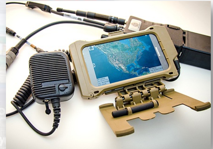
The Wave Relay Android Kit from Persistent Systems pairs Android devices with Wave Relay, a radio system that provides a secure Mobile Ad Hoc Network (MANET)
